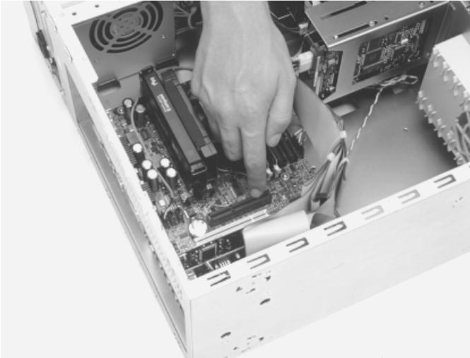
2. Remove the metal slot cover. Save the screw to secure the graphics card later.
