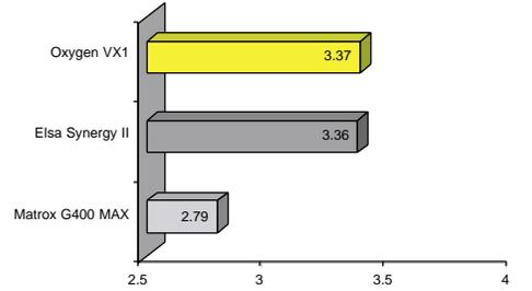
Test Platform: 1000 MHz Pentium III AGP4X, 512 Mb of RAM, 1280x1024@75Hz refresh rate
