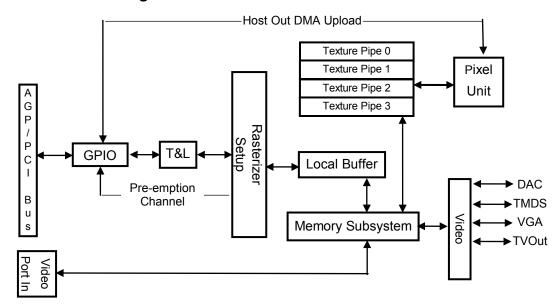
Figure 1.1 Chip-level Block Diagram
