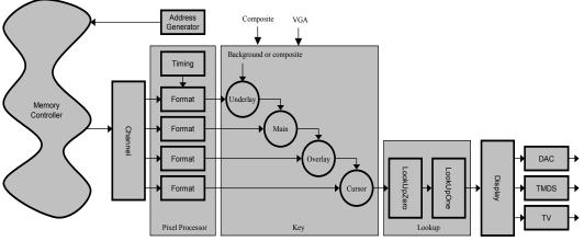
All channels are identical except that they have a fixed stacking order (cursor over overlay over main over underlay) and the main and overlay channels can be run in stereo mode.
