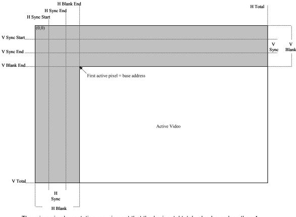
There is an implementation requirement that the horizontal total value be no less than 4 and that there must be at least one line of vertical blank.
