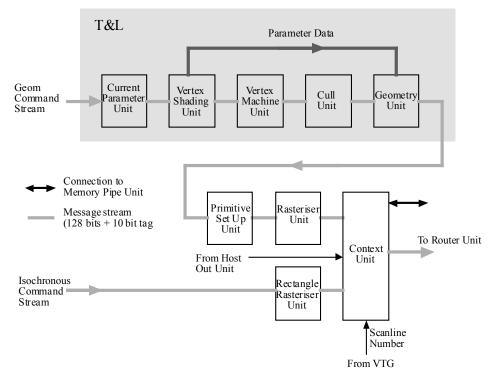
Figure 1.2 Transformation and Lighting Block Diagram
