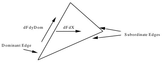
Figure 5.26 Fog Interpolation Over A Triangle
