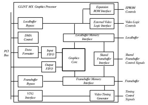
Figure 2.1 High level blocks in the GLINT architecture
