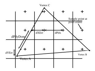
The vertices are sorted into Y order and the dominant edge is AC. Scan conversion will start at vertex A and proceed upwards. The origin is bottom left.
