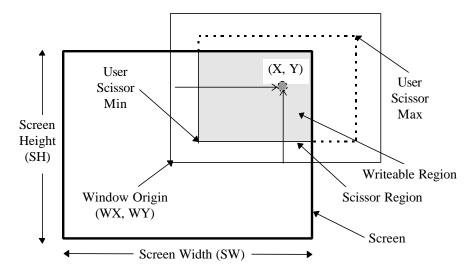
Figure 5.12 Screen Scissor and User Scissor Tests
