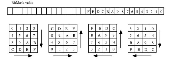
Figure 5.9 Relationship between Bitmask and Scanning Directions
