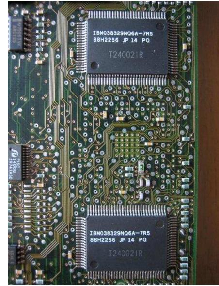
Located in the back of the card2starsPQFPpackage,IBM SGRAMmemory, chip size1 MB,7.5ns, the maximum operating frequency of133MHz, specifically forPERMEDIA 2 Vgraphics chips to use.
