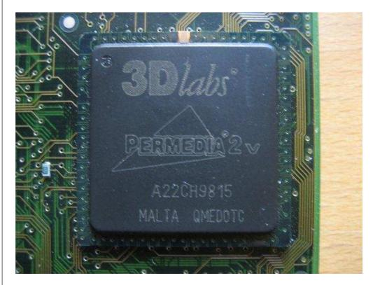
The only use of block graphicsBGApackage3Dlabs PERMEDIA 2Vchip, this card is onl y used in2Dthe basic display.PERMEDIA 2 of the 2D performance is certainly outstandi
