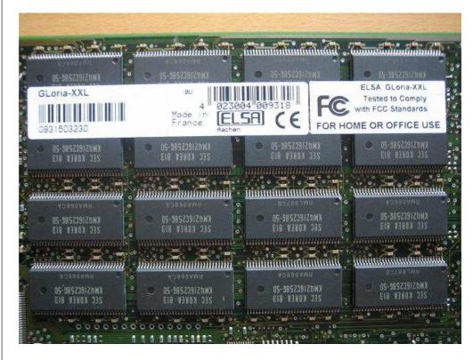
16MBframe buffer, from both sides of the16films threestars256K X 16 VIDEO RAMco mposed of single size512KB,50ns, used to storeframe bufferdata. Memory is also posted on theELSAmodel label, you can see in the abovegraphicsorigin is France.
